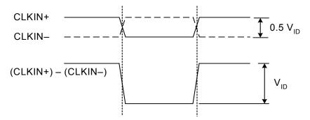
B. Operation with Differential Clock Inputs
