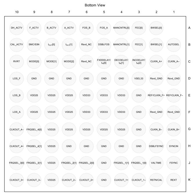
Figure 15. Si5364 Pin Configuration (Bottom View)
