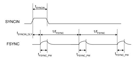
Figure 3. SYNCIN and FSYNC Timing
