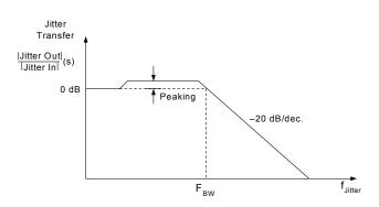
Figure 10. PLL Jitter Transfer Mask/Template
