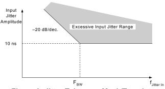
Figure 9. Jitter Tolerance Mask/Template
