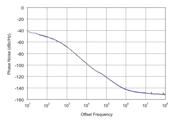
Figure 7. Typical Si5364 Phase Noise (CLKIN = 19.44 MHz, CLKOUT = 622.08 MHz, and Loop BW = 800 Hz)
