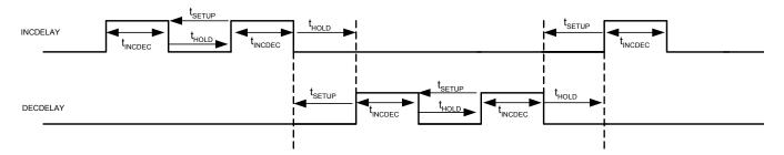
Figure 5. Clock Input to Clock Output Delay Adjustment (Pin Control)
