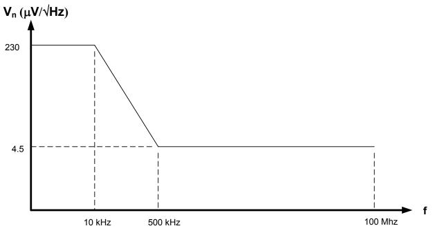
Figure 14. Power Supply Noise Tolerance Mask
