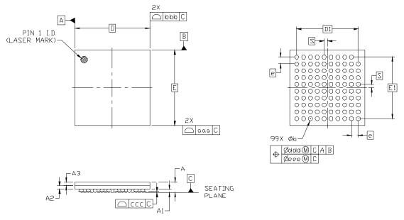
Figure 17. 99-Ball Plastic Ball Grid Array (PBGA)
