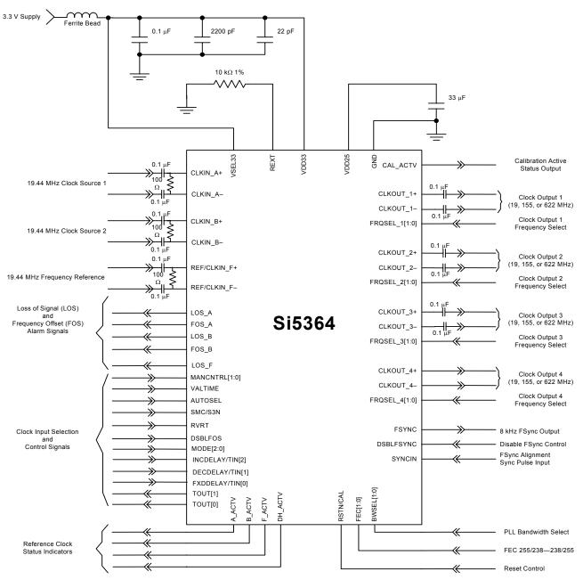
Figure 8. Si5364 Typical Application Circuit (3.3 V Supply)
