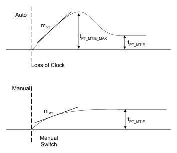
Figure 11. Phase Transient Specification
