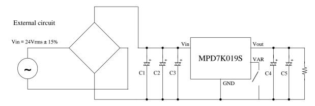
C1,C2,C3: 1000μF/50V Low Impedance Aluminum Electrolytic Capacitor (EKZE500EC3102ML25S NIPPON CHEMI-CON)
