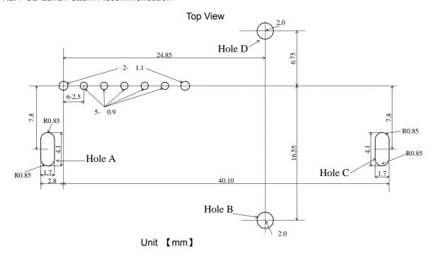
Metal case is connected to GND. So hole A,B,C and D should be connected to GND. The Area indicated find is allowed no pattern or only GND pattern.
