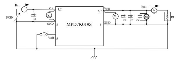
C1 : 1000μF/50V Low Impedance Aluminum Electrolytic Capacitor (ZL series : Rubycon) C2,C3 : 1000μF/16V Low Impedance Aluminum Electrolytic Capacitor (EKZE160ETD102MJ20S NIPPON CHEMI-CON)
