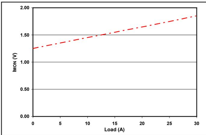
Figure 9: I<sub>mon</sub> pin voltage vs. load current at 24V input and 13.8V output. Load capacitance: 100µF electrolytic cap. C option only.
