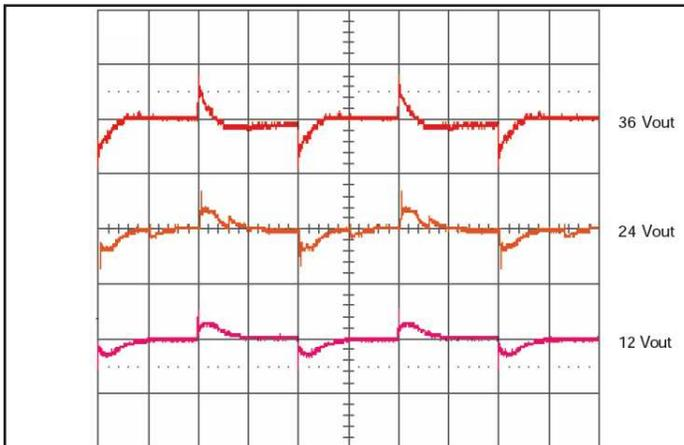
Figure 11: Output voltage response for 24V input; 12V, 24V, 36V output to step-change in load current (50-75-50% of I<sub>out</sub> max; di/dt=0.1A/µs). Load cap: 100µF, 100mΩ ESR tant, Ch 1-3: Vout (2V/div);(5ms/div).
