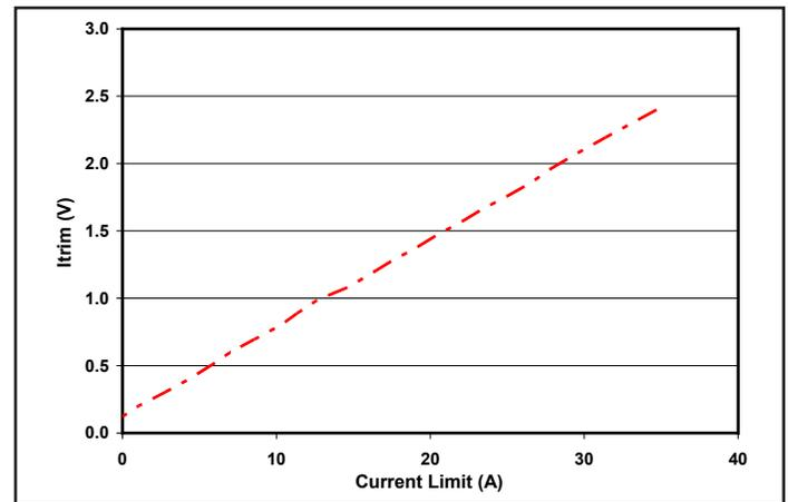
Figure 10: Current limit vs. I<sub>trim</sub> pin voltage with 24V input and 13.8V output. Load capacitance: 100µF electrolytic cap. C option only.
