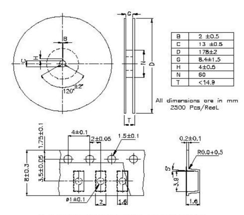
Accumulated pitch tolerance is  $\pm 0.2~\mathrm{mm}$  over ID pitches 8-mm Carrier tape for Quadro MELF — LS34 PACKAGE All dimensions are in mm
