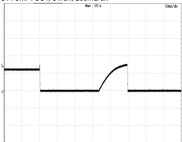
Figure 6: Output over voltage protection at 48V in , 24A I out CH1:VOUT, 10V/div, 50mS/div
