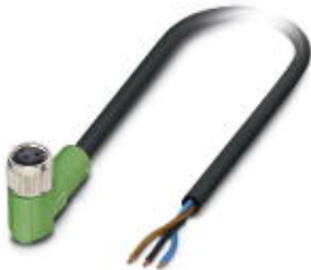
Sensor/Actuator cable, 3-position, PVC, Black RAL 9005, Free cable end, on Socket angled M8, Cable length: 2 m
