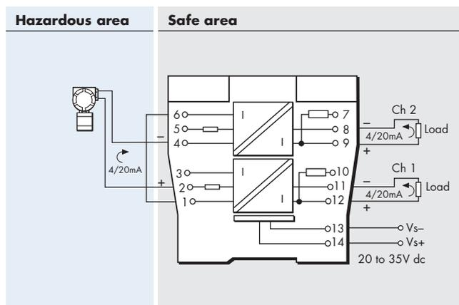
The MTL5544 can also be used to drive two safe-area loads from a single 2-wire transmitter (i.e. 1 in, 2 out) by interconnecting the input channels as shown in the diagram here.
