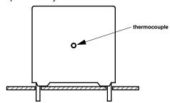
The temperature is measured in unloaded (T<sub>amb</sub>) and maximum loaded condition (T<sub>c</sub>).
