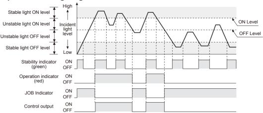
\*\*The waveforms of operation indicator, job indicator, and control output are the state of operation for Light ON, but in case of Dark ON, it is opposite operation against Light ON mode.
