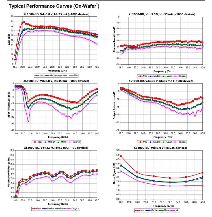
Note [1] Measurements – On-Wafer data has been taken using bias conditions as shown. Measurements are referenced 150 um in from RF In/Out pad edge. For optimum performance M/A-COM-Tech T-pad transition is recommended. For additional information see the M/A-COM-Tech "T-Pad Transition" application note.
