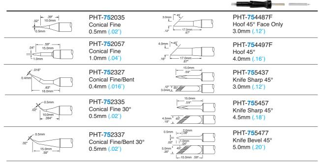
75 = 750 Series for most standard applications. 65 = 650 Series also available for temperature sensitive applications. To order this series, replace 75 with 65.
