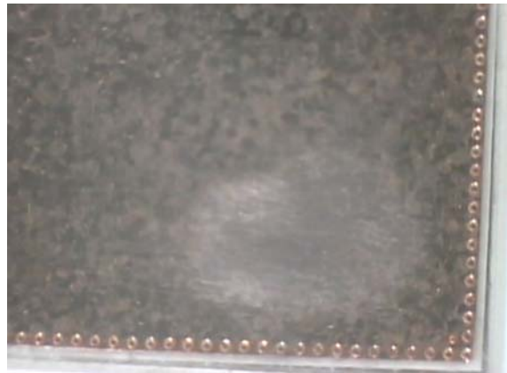
Fig. 5: Acceptable reworked MiniSKiiP bottom surface
