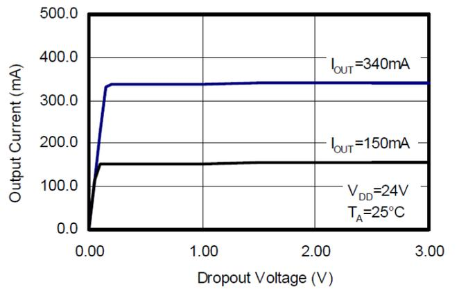
**Figure 4. Output Current vs. Dropout Voltage**
