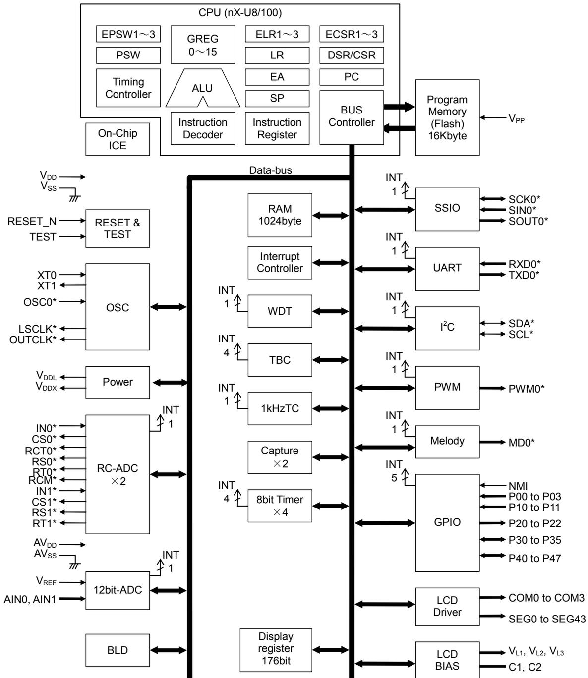
**Figure 2 ML610Q412 Block Diagram**
