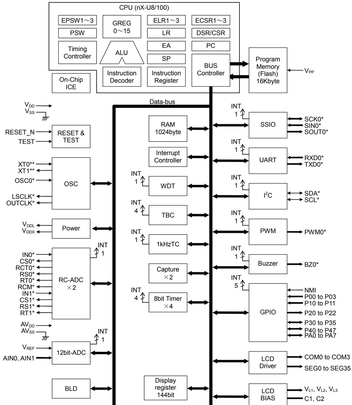
Figure 1 ML610Q411/ML610Q415 Block Diagram
