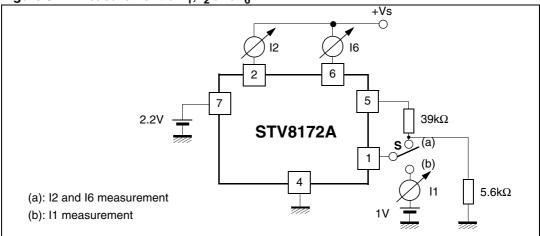
Figure 4. Measurement of V<sub>5H</sub>
