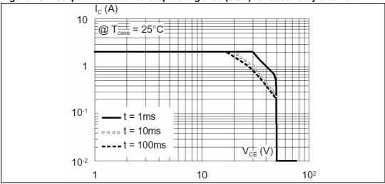
The diagram has been arbitrarily limited to max I0 (2A).
