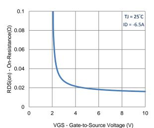
3. On-Resistance vs. Gate-to-Source Voltage
