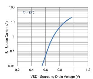
4. Drain-to-Source Forward Voltage
