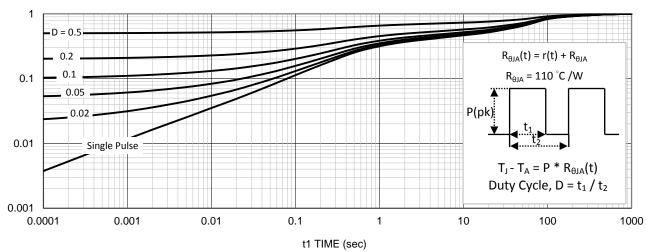
11. Normalized Thermal Transient Junction to Ambient
