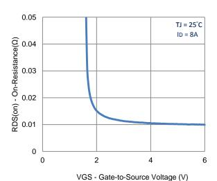
3. On-Resistance vs. Gate-to-Source Voltage
