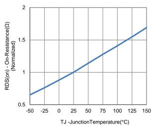
8. Normalized On-Resistance Vs **Junction Temperature**
