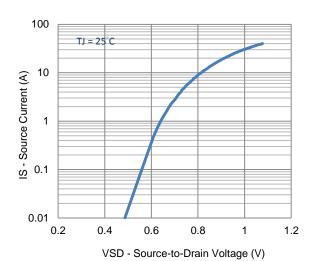
4. Drain-to-Source Forward Voltage
