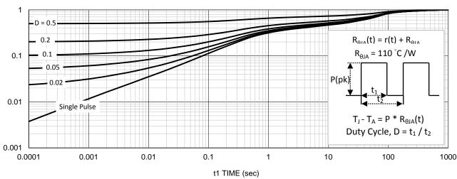
11. Normalized Thermal Transient Junction to Ambient
