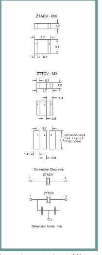
The terminations of the ZTACV and ZTTCV series ceramic resonator are Pb free. Pb may be contained in the ceramic resonator element of this device and is exempted via item 7 of the RoHS annex. This ceramic resonator series is considered RoHS compliant.
