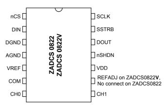
Figure 3 Package Pin Assignment for ZADCS0822 & ZADCS0822V
