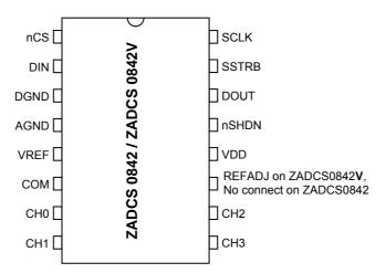
Figure 2 Package Pin Assignment for ZADCS0842 & ZADCS0842V
