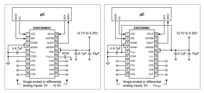
Figure 4: Basic application schematic for ZADCS0882V
