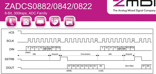
Figure 13: 16-Clock External Clock Mode Conversion
