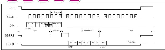
Figure 11: 24-Clock External Clock Mode Timing ( $f_{SCLK} \le 3.3MHz$ )
