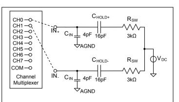
Figure 9: Equivalent input circuit during sampling
