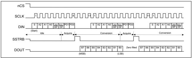
Figure 14: 11-Clock External Clock Mode Conversion
