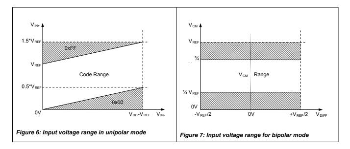
The voltage at IN<sub>-</sub> can range from -0.2V ...  $\frac{1}{2}$  V<sub>REF</sub> without limiting the Code Range, assuming the fore mentioned VDD condition is true. See also Figure 6 for input voltage ranges in unipolar conversion mode.
