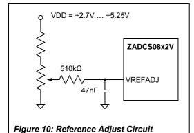
Basic ZADCS08x2 devices do not contain the internal bandgap or the VREF buffer. An external reference must be supplied all the time at VREF.
