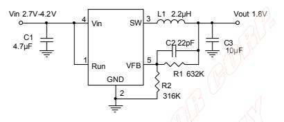
Fig.1 Basic Application Circuit with LSP3100 adjustable version
