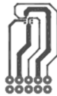
b. 415\text{ }^\circ\text{C/W} when mounted on a minimum pad of 2 oz copper.
