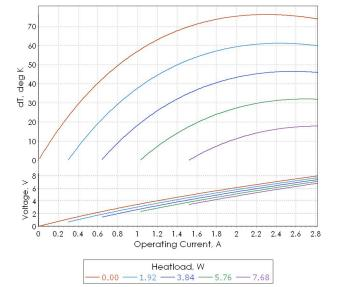
**Note**: Performance data is specified for optimal conditions (TEC hot side is stabilized at ambient temperature). Heatsink thermal resistance is not included into estimations. Use TECCad Software for estimations under different conditions.
