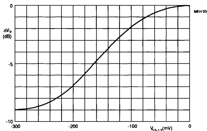
Fig.8 High Cut Control (HCC) at  $f_{\text{mod}} = 10 \text{ kHz}$ .
