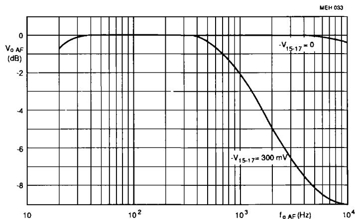
Fig.7 High Cut Control (HCC) as a function of audio frequency.
