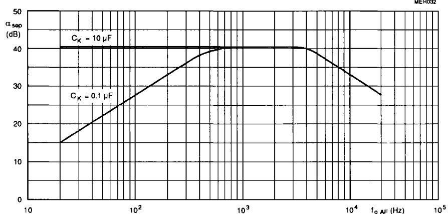
Fig.6 Channel separation as a function of audio frequency.
