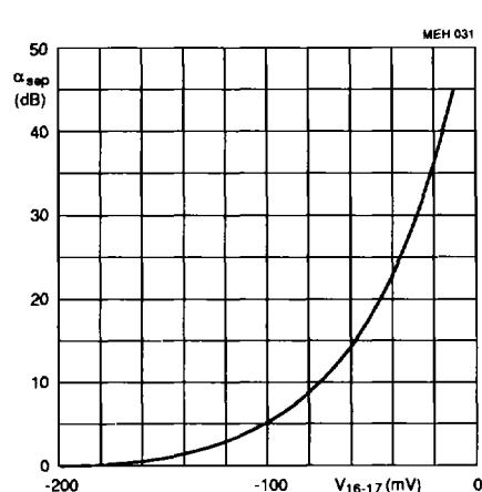
Fig.5 Stereo blend characteristic (SNC).
