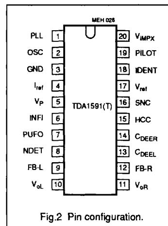
Fig.2 Pin configuration.
