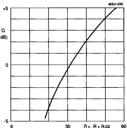
Fig.4 Over all signal gain as a function of feedback resistors  $R_2$  and  $R_3$  ( $R_1 = 150$   $k\Omega$ ).
