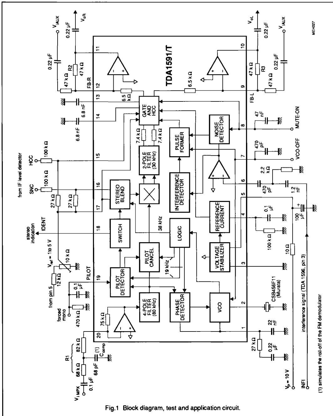
Fig.1 Block diagram, test and application circuit.
