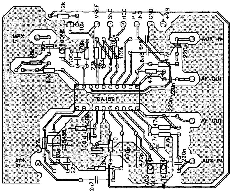
Fig.9 TDA1591(T) testboard (component side).
