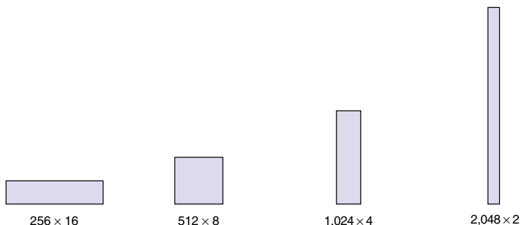
Figure 5. FLEX 10KE EAB Memory Configurations
