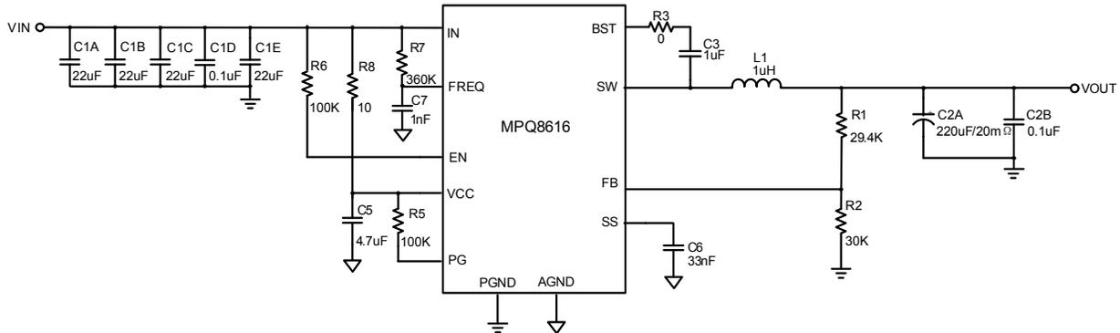
**Figure 13 — Typical Application Circuit with No External Ramp**
