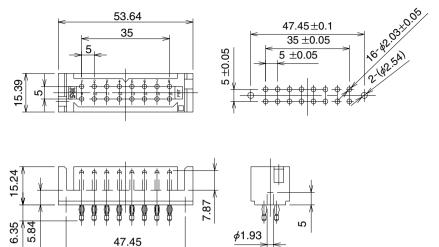
Copper plating thickness :  $70 \pm 10 \mu m$ Solder plating thickness : 5 to 10  $\mu$ m Board thickness : 3.2 mm min. Fasten to the board being sure to use (American type) #2 tapping screws.
