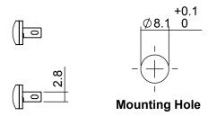
Anode termination indicated by red sleeve. Mounting hole to be clean and burr free.
