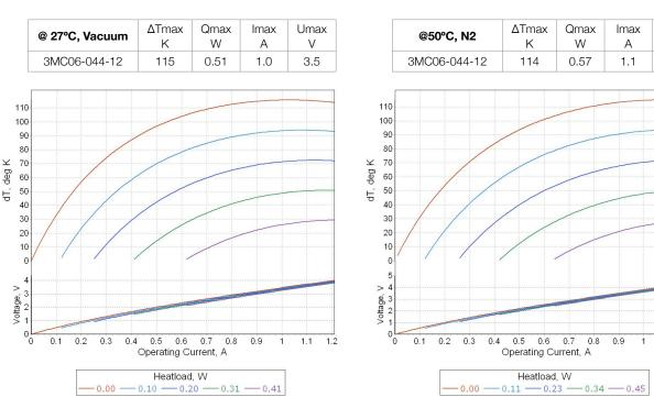
**Note**: Performance data is specified for optimal optimal conditions (TEC hot side is stabilized at ambient temperature). Heatsink thermal resistance is not included into estimations. Use TECCad Software for estimations under different conditions.
