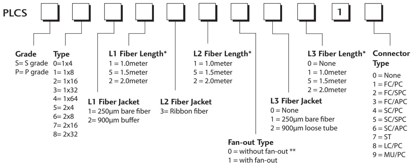
\* The tolerance of fiber length is +/-0.1m.
