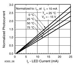
Fig. 4 - Normalized Servo Photocurrent vs. LED Current and Temperature
