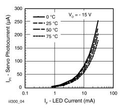
Fig. 3 - Servo Photocurrent vs. LED Current and Temperature
