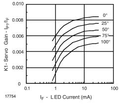
Fig. 5 - Servo Gain vs. LED Current and Temperature
