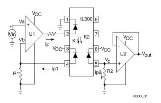
Fig. 1 - Typical Application Circuit
