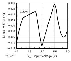
Fig. 15 - Linearity Error vs. Input Voltage
