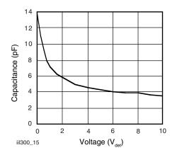
Fig. 10 - Photodiode Junction Capacitance vs. Reverse Voltage
