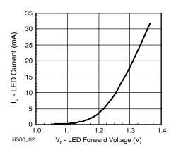
Fig. 2 - LED Forward Current vs. Forward Voltage
