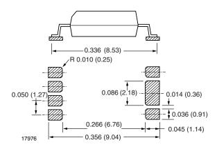
Fig. 5 - 8 Pin PCMCIA, Heat Sink
