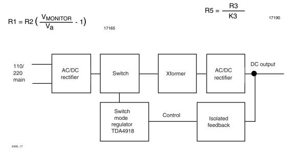
Fig. 12 - Switching Mode Power Supply
