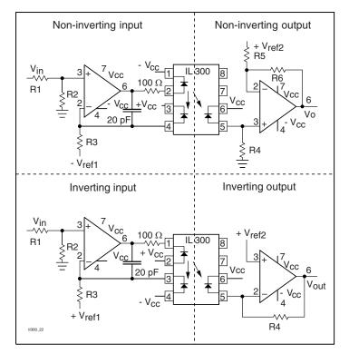
Fig. 17 - Non-inverting and Inverting Amplifiers
