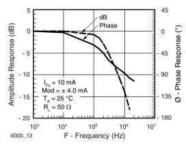
Fig. 8 - Amplitude and Phase Response vs. Frequency
