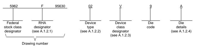
A.1.2.1 <u>RHA designator</u>. Device classes Q and V RHA identified die meet the MIL-PRF-38535 specified RHA levels. A dash (-) indicates a non-RHA die.
