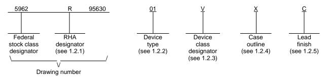
1.2.1 <u>RHA designator</u>. Device classes Q, T and V RHA marked devices meet the MIL-PRF-38535 specified RHA levels and are marked with the appropriate RHA designator. A dash (-) indicates a non-RHA device.
