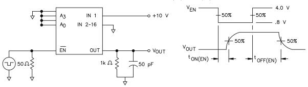
FIGURE 5. Test circuits and waveforms for ac levels.
