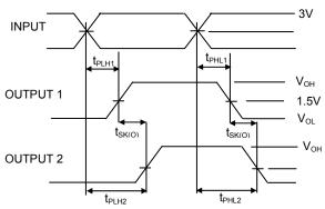
$t_{SK(O)}$  = |  $t_{PLH2}$  -  $t_{PLH1}$  | or |  $t_{PHL2}$  -  $t_{PHL1}$  |
