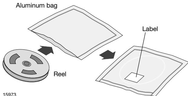
After more than 72 h under these conditions moisture content will be too high for reflow soldering.
