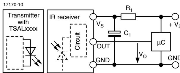
The external components R<sub>1</sub> and C<sub>1</sub> are optional to improve the robustness against electrical overstress (typical values are R<sub>1</sub> = 100 Ω, C<sub>1</sub> = 0.1 μF).
