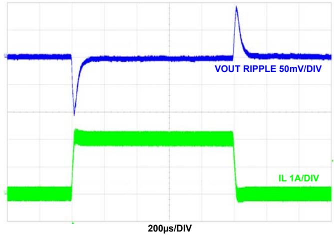
**FIGURE 46. LOAD TRANSIENT**
