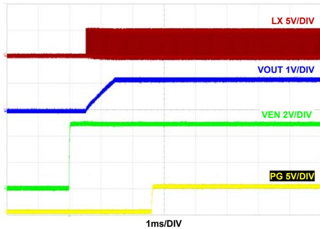
FIGURE 25. START-UP AT 2A LOAD
