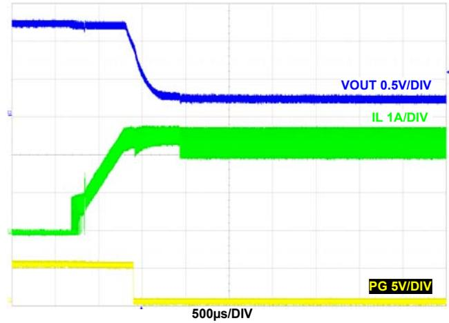
**FIGURE 48. OVERCURRENT PROTECTION**
