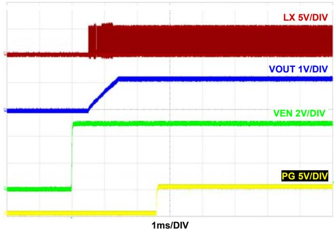
FIGURE 22. START-UP AT NO LOAD
