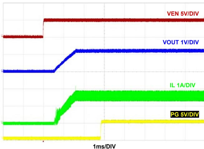
FIGURE 31. START-UP AT 1.5A LOAD
