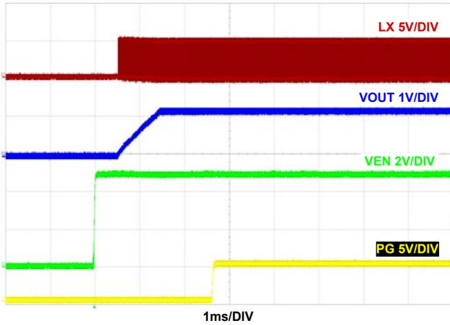
FIGURE 27. START-UP AT 2A LOAD
