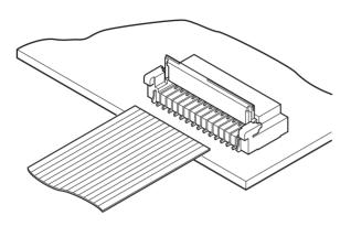
Non-ZIF type connector for FPC's, with only 2.25mm height when mounted on the PC board. Temporary retention mechanism and flip-lock device provide good operational efficiency.
