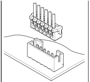
The KR connector features a mounting height as low as 6.9mm and a thickness as thin as 4.8mm (for top entry type). It is suitable for interconnection of a wide range of electronic equipment such as VCRs. video cameras, car stereo systems and communication equipment.
