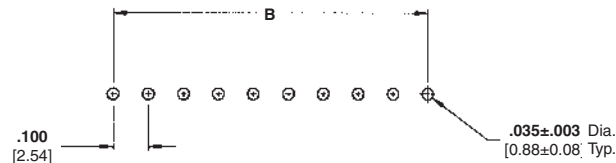
Recommended PC Board Hole Layout (for .062 [1.57] thick PC board)
