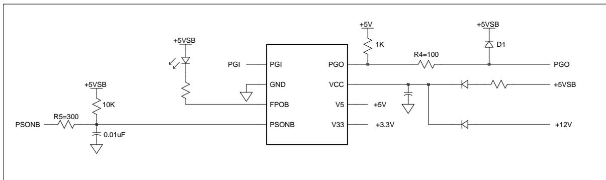
NOTE1 : The series resistor R5 at PSONB can not be omitted. ( R5 = 300 Ω is suggested )
