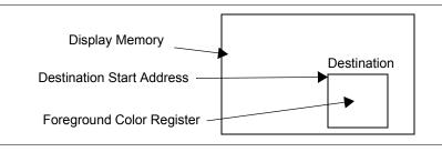
Figure 16-4: Solid Fill BitBLT Data Flow
