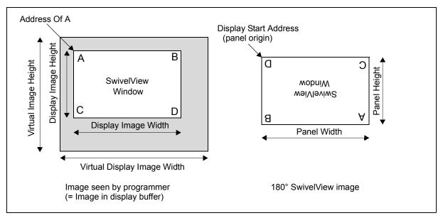
Figure 14-2: Relationship Between The Screen Image and the Image Refreshed in 180° SwivelView.
