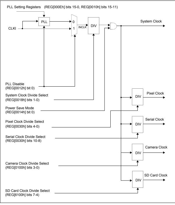
Figure 9-1: Clock Diagram
