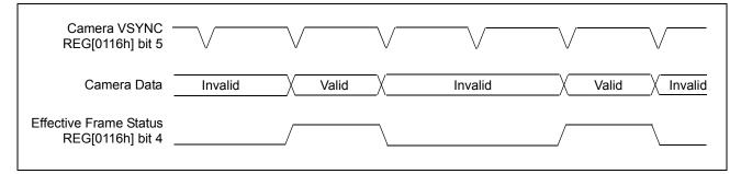
Figure 10-1: Effective Frame Status Bit Example
