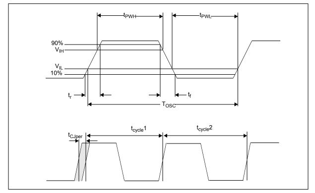
Figure 7-1: Clock Input Requirements (PLL)
