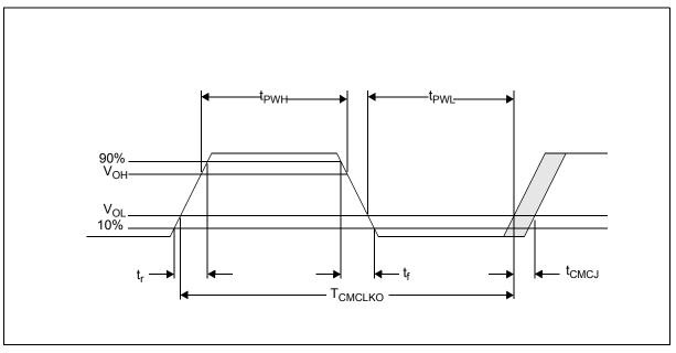
Figure 7-42: Camera Clock Output Timing
