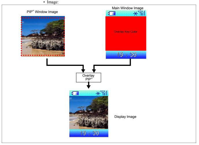
Figure 8-5: Main Window, PIP<sup>+</sup> Window, and Overlay Display
