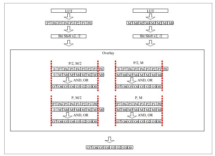
The following table shows the resulting  $PIP^+$  window color when overlay is combined with the  $PIP^+$  Window Bit Shift and the Main Window Bit Shift functions.
