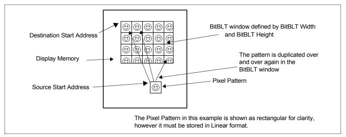
Figure 16-3: Pattern Fill Drawing
