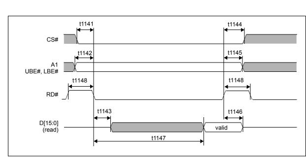
Figure 7-20: Indirect 80 Type 1 Interface Read Cycle Timing (No Wait Mode)
