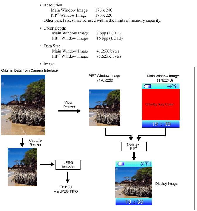
Figure 8-9: Main Window, PIP<sup>+</sup> Window, Overlay, and JPEG
