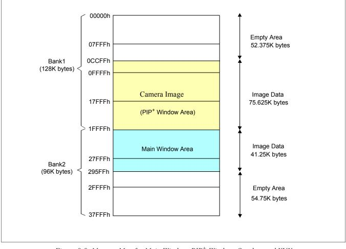
Figure 8-8: Memory Map for Main Window, PIP<sup>+</sup> Window, Overlay, and YUV
