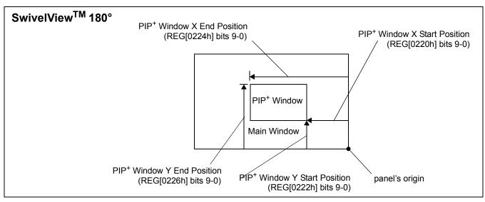
*Figure 15-3: PIP*<sup>+</sup> *with SwivelView 180° Enabled*
