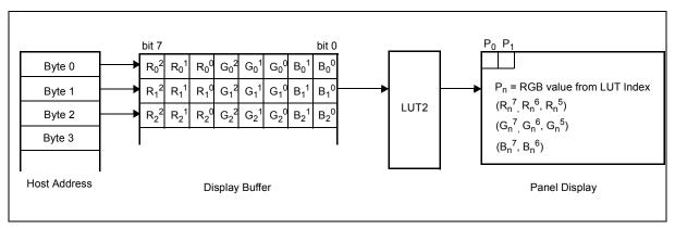
Figure 13-2: LUT2 for 8 Bpp Mode
