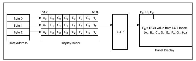
Figure 13-1: LUT1 for 8 Bpp Mode
