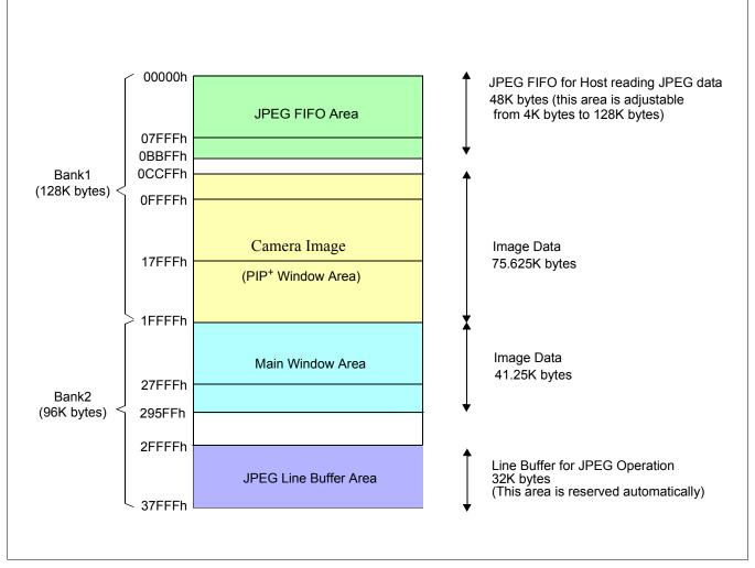
Figure 8-10: Memory Map for Main Window, PIP<sup>+</sup> Window, Overlay and JPEG
