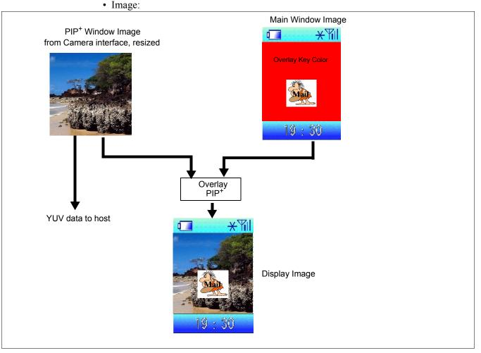
Figure 8-7: Main Window, PIP<sup>+</sup> Window, Overlay, and YUV
