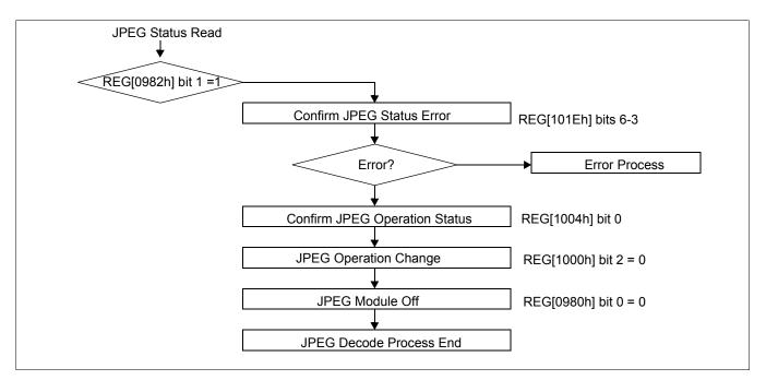
Figure 19-11: JPEG Decoding Process (6 of 6)
