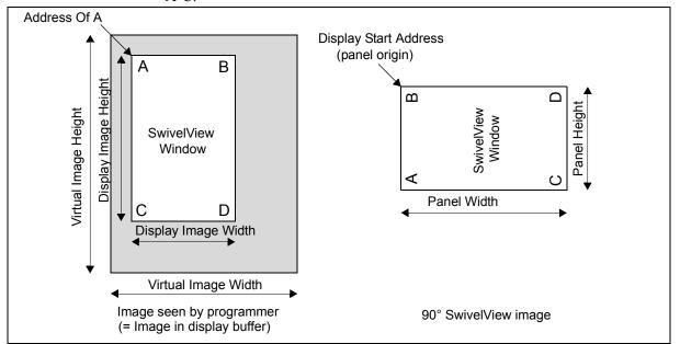
Figure 14-1: Relationship Between The Screen Image and the Image Refreshed in 90° SwivelView.
