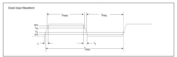
Figure 7-2: Clock Input Requirements (PLL bypassed)
