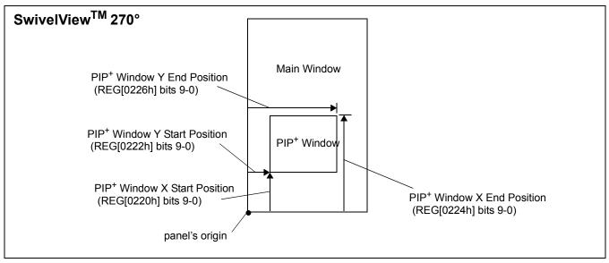
*Figure 15-4: PIP*<sup>+</sup> *with SwivelView 270° Enabled*
