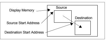
Figure 16-2: Move BitBLT data flow
