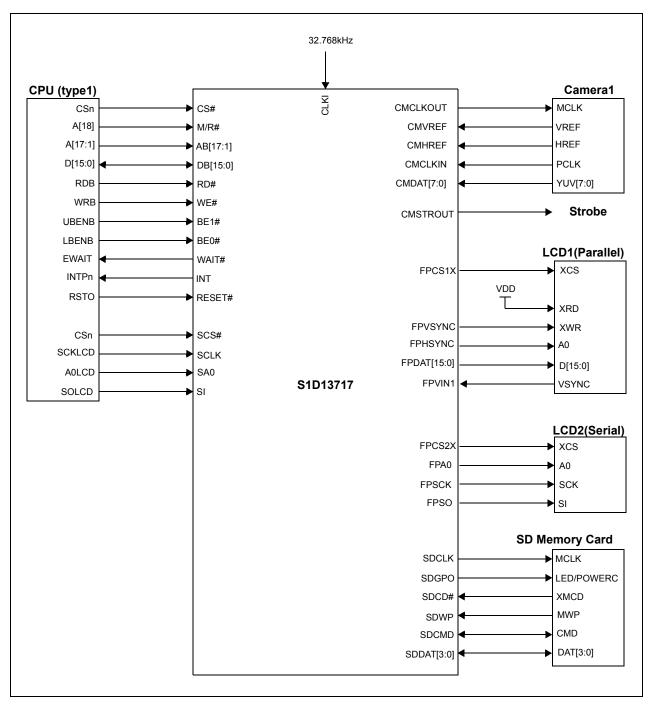
Figure 3-3: S1D13717 System Diagram 3
