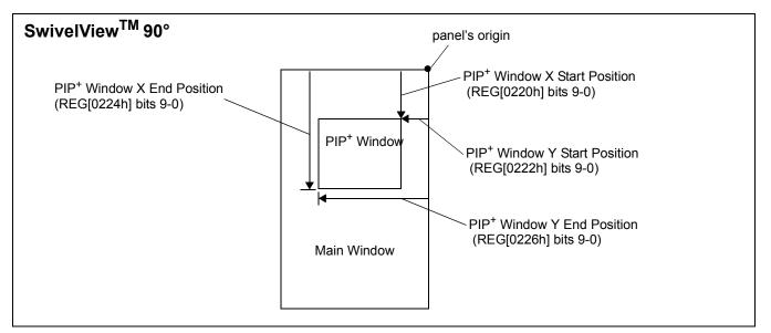
*Figure 15-2: PIP*<sup>+</sup> *with SwivelView 90° Enabled*
