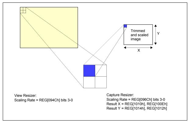
Figure 17-2: Scaling Example (1/2 Scaling)
