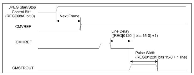
Figure 20-1: Strobe Signal Output Timing
