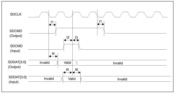
Figure 7-44: SD Memory Card Access Timing
