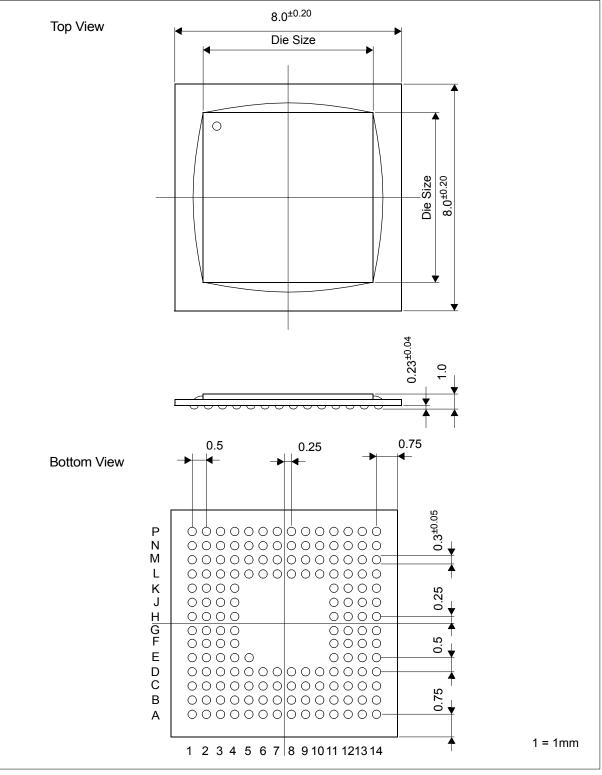
Figure 23-1: S1D13717 FCBGA-161 Pin Package
