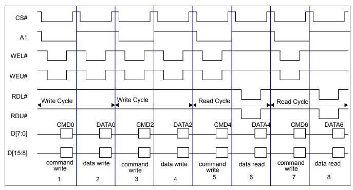
Figure 22-1: Register Read/Write" Example Sequence
