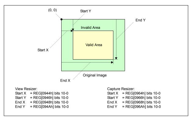
Figure 17-1: Trimming Function
