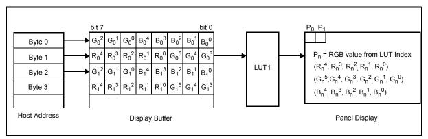
Figure 13-3: LUT1 for 16 Bpp Mode
