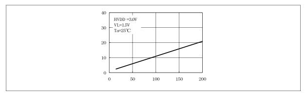
Figure 7-40: Fall Time V.s. Capacitance  $(C_L)$
