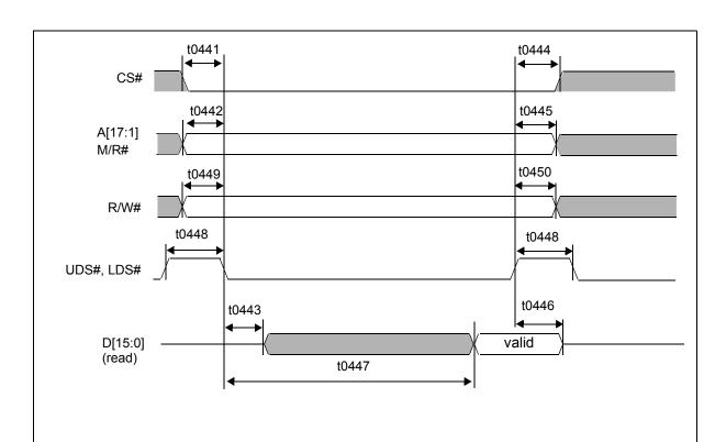
Figure 7-17: Direct 68 Interface Read Cycle Timing (No Wait Mode)
