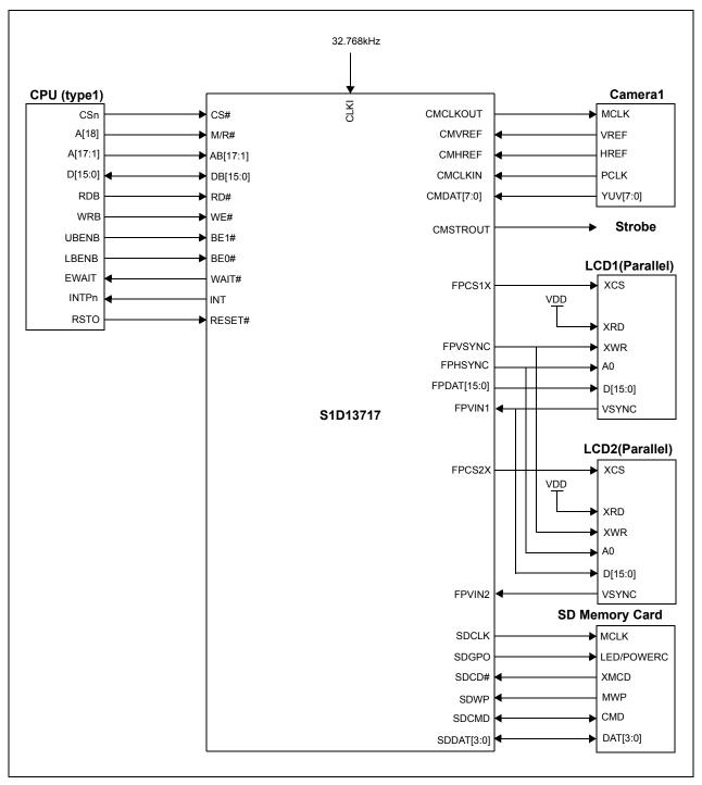
Figure 3-4: S1D13717 System Diagram 4
