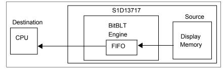
Figure 16-1: Read BitBLT Data Flow
