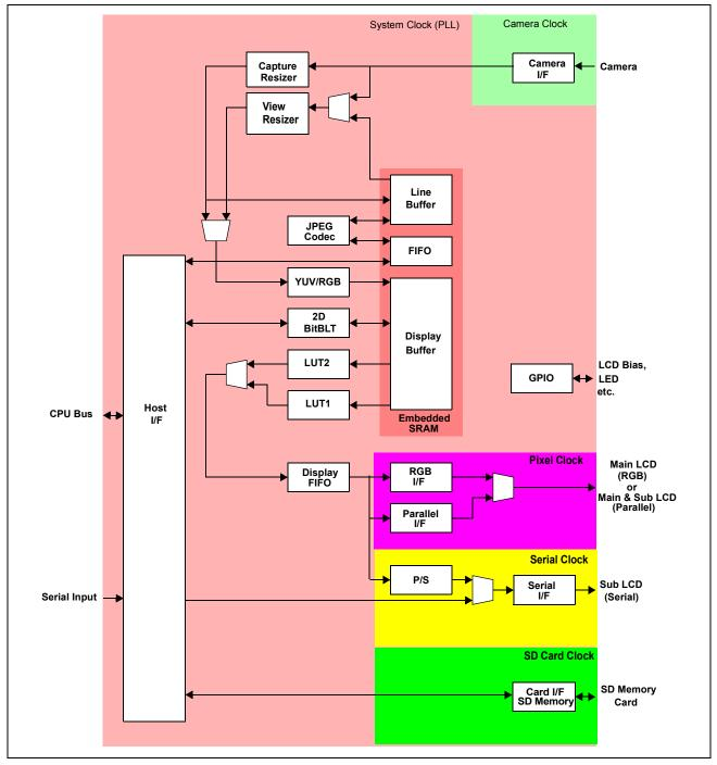
Figure 4-1: S1D13717 Block Diagram
