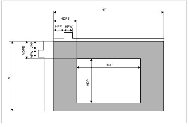
Figure 7-30: Generic TFT Panel Timing
