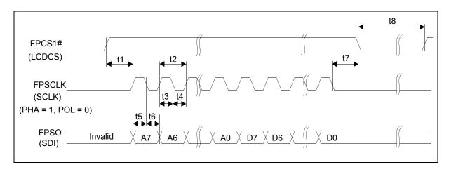
Figure 7-36: LCD1 uWIRE Serial Interface Timing
