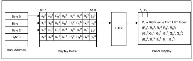
Figure 13-4: LUT2 for 16 Bpp Mode
