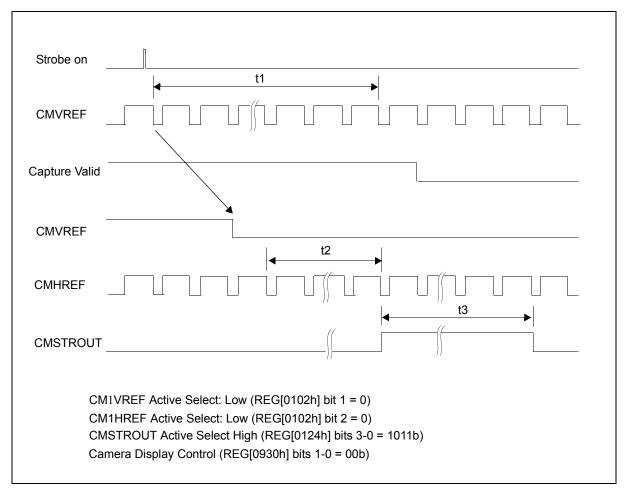
Figure 7-43: Strobe Control Output Timing
