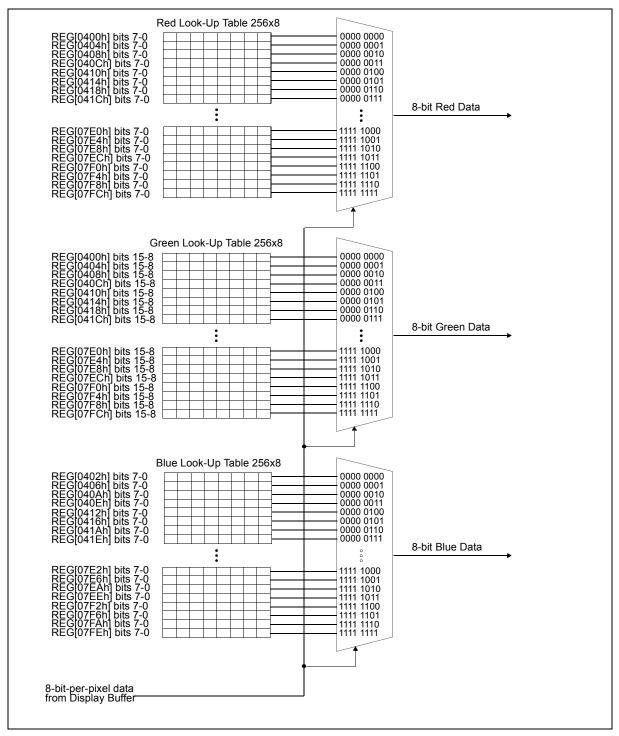
Figure 12-1: LUT1 (Main Window) for 8 Bpp Architecture
