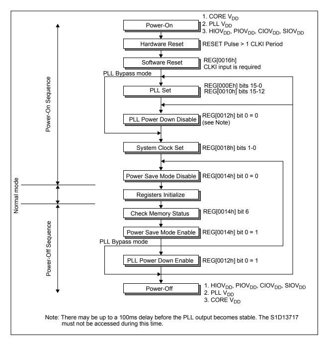
Figure 11-1: Power-On/Power-Off Sequence
