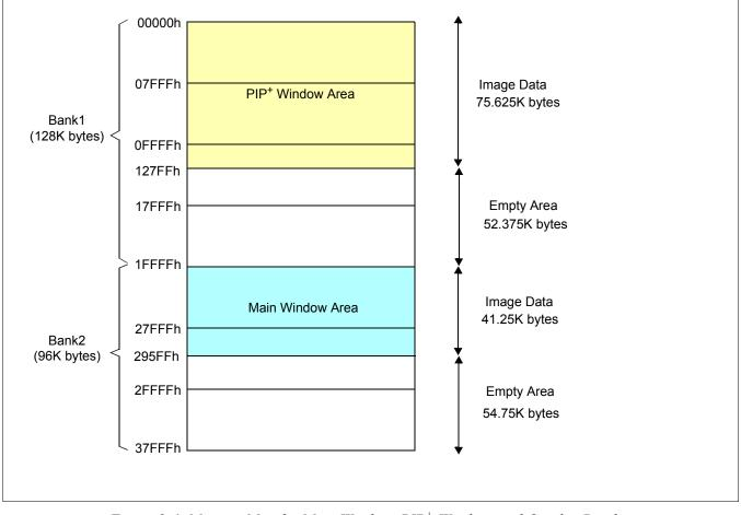
Figure 8-6: Memory Map for Main Window, PIP<sup>+</sup> Window, and Overlay Display
