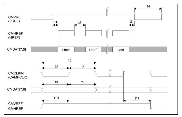
Figure 7-41: Camera Interface Timing
