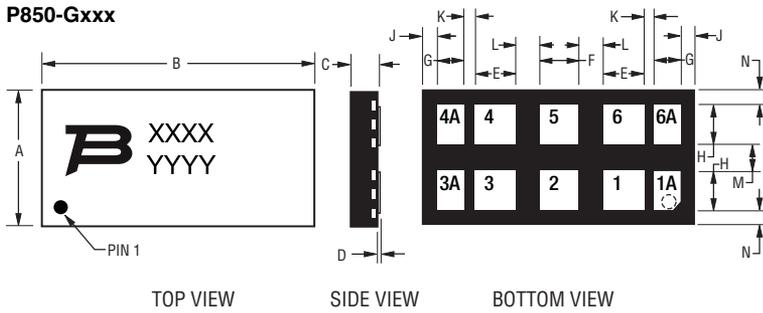
Pads 1A and 1 are internally connected; the same for pads 3A with 3, 4A with 4, and 6A with 6. This allows for one PCB layout to accommodate the P500 or P850.
