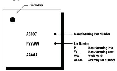
Note: Prior to production release, the marking will be 'E5007'. After the completion of Avago qualification testing and production release, the marking will revert to 'A5007'.
