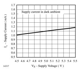
Figure 10. Supply Current vs. Supply Voltage
