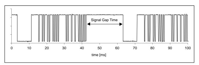
Figure A: Data Signal (Output of IR Receiver) with a Signal Gap Time of 20ms
