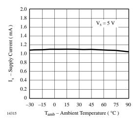
Figure 8. Supply Current vs. Ambient Temperature
