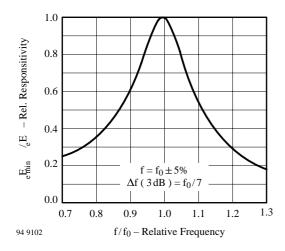
Figure 1. Frequency Dependence of Responsivity
