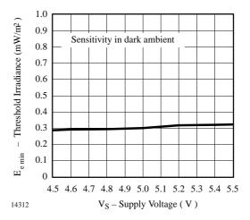
Figure 5. Sensitivity vs. Supply Voltage
