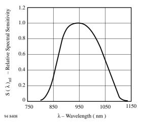
Figure 11. Relative Spectral Sensitivity vs. Wavelength
