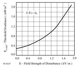
Figure 3. Sensitivity vs. Electric Field Disturbances
