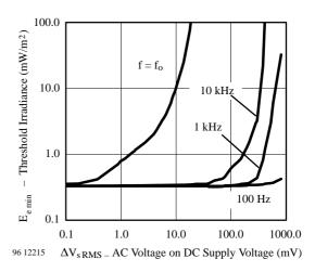
Figure 4. Sensitivity vs. Supply Voltage Disturbances
