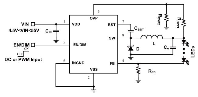
Figure 3: White LED Driver Step-Down Application
