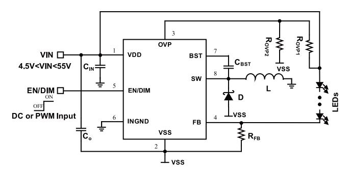
Figure 5: White LED Step-Up Driver Application
