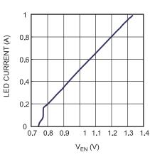
**Analog Dimming Curve**
