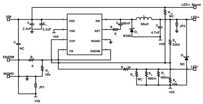
Figure 6: Design Example White LED Driver;
