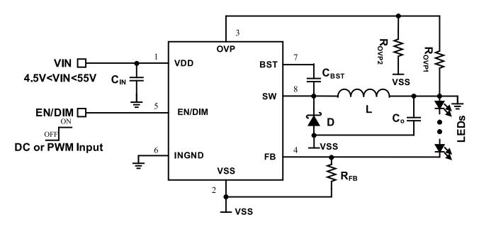
Figure 4: White LED Driver Step-Up/Down Application
