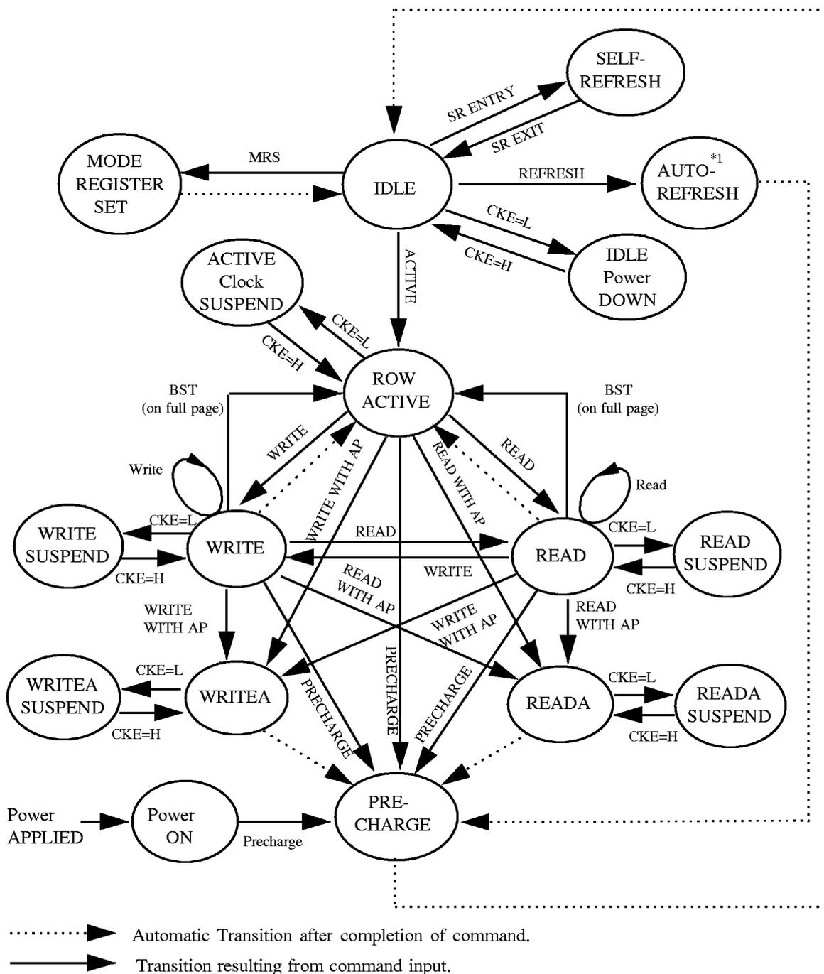
Note: 1. After the auto-refresh operation, Precharge is performed automatically and enter the IDLE state.
