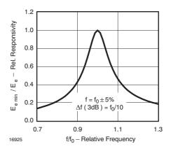
Figure 5. Frequency Dependence of Responsivity
