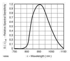
Figure 11. Relative Spectral Sensitivity vs. Wavelength
