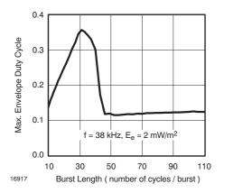
Figure 9. Max. Envelope Duty Cycle vs. Burstlength
