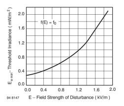
Figure 8. Sensitivity vs. Electric Field Disturbances
