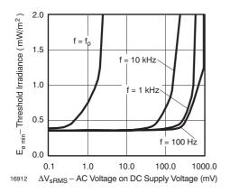
Figure 7. Sensitivity vs. Supply Voltage Disturbances
