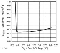
Figure 12. Sensitivity vs. Supply Voltage
