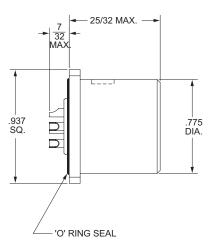
GC729 RECEPTACLE Rigid contacts, solder terminals, mates with
