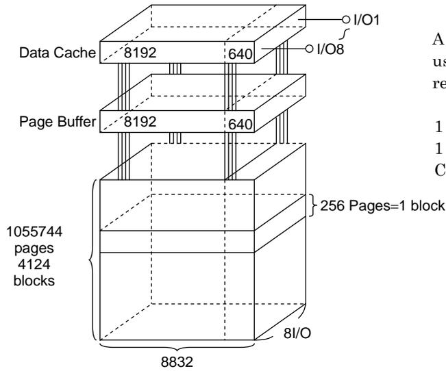
A page consists of 8832 bytes in which 8192 bytes are used for main memory storage and 640 bytes are for redundancy or for other uses.
