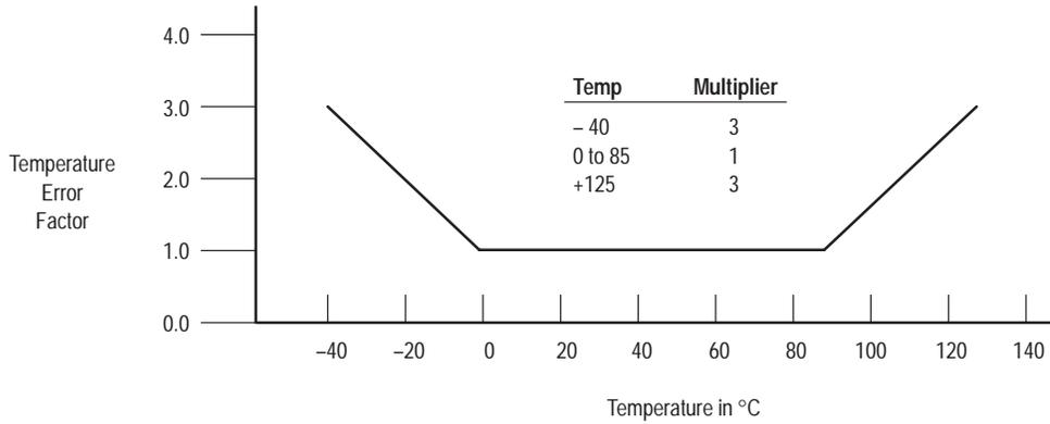
NOTE: The Temperature Multiplier is a linear response from 0° to -40°C and from 85° to 125°C.
