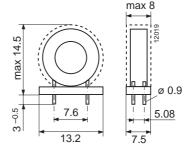
Fig. 11 Common mode choke LP183, weight 7 g
