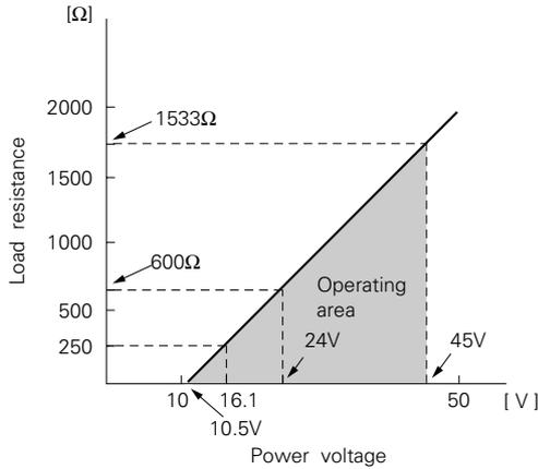
Note: For communication with FXW, min. of 250 Ω required.
