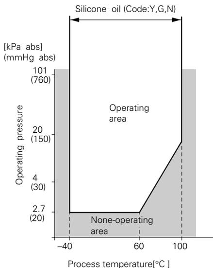
Fig. 1 Relation between process temperature and operating pressure
